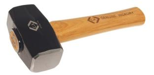
Features & Benefits  $\sim$  Drop forged high carbon steel head  $\sim$  Hardened & tempered for superior strength and durability  $\sim$  Black lacquered to protect against corrosion  $\sim$  Tough hickory shaft to withstand high impact applications  $\sim$  Weight: 1135 g / 2.1/2lb
